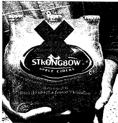
Pic 1: Incorrect Shrink
